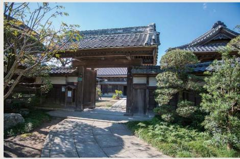
The front gate is a full-fledged yakui-mon gate constructed in the end of the Edo Period. These are characterized by having two main pillars and two support pillars in the rear that undergird a gabled roof.
